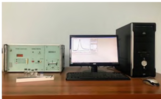
"Iskovich" thermal desorption surface ionization measuring complex
