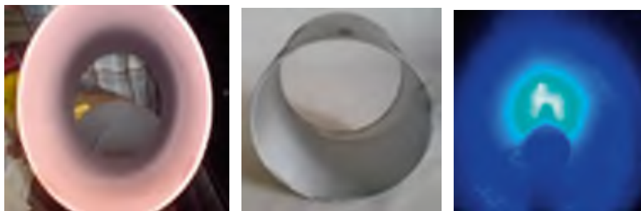
Technology of electric arc cleaning and application of protective coating on the inner surface of metal pipes.
