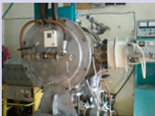
Technological installation for ion-plasma deposition and synthesis by ion bombardment of strengthening titanium nitride coatings.
