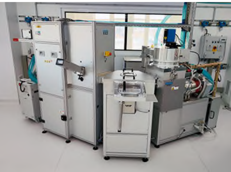
Growth setup – cluster of atomic layer, chemical and plasma-enhanced chemical vapor deposition (PEALD, PECVD) with vacuum loading lock
