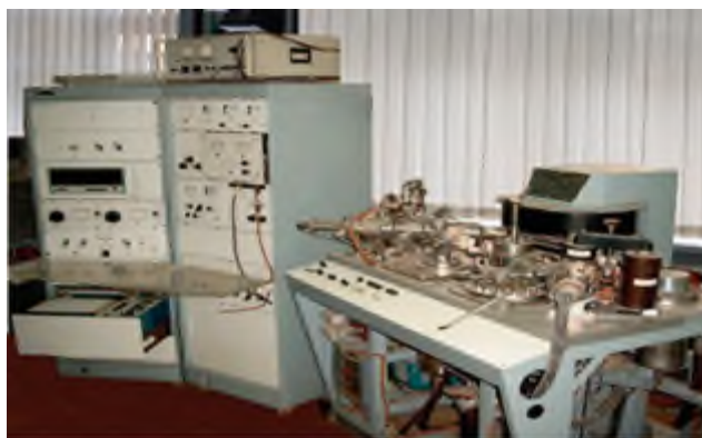
Mass spectrometer MI-1201V, modernized for studying surface ionization
