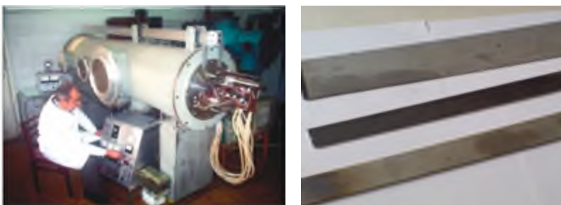
Technological installation for electric arc cleaning of metal products
